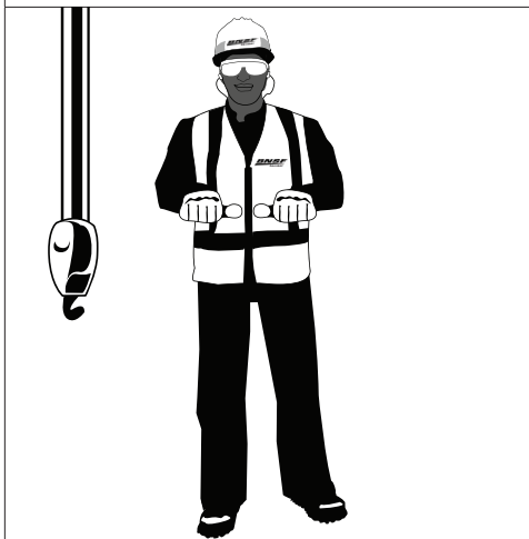
RETRACT BOOM (Telescoping Booms): Both fists in front of body with thumbs pointing toward each other.
