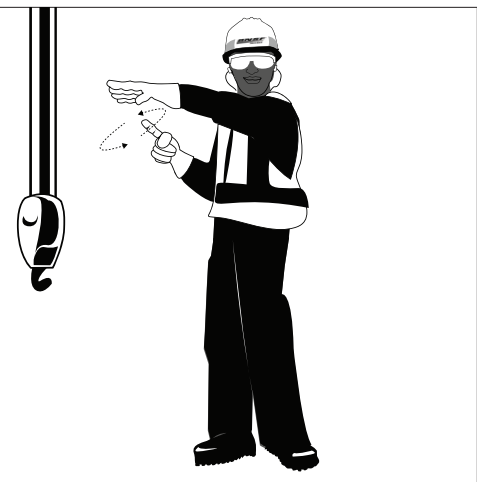
MOVE SLOWLY: Use one hand to give any motion signal and place other hand motionless in front of hand giving the motion signal.
