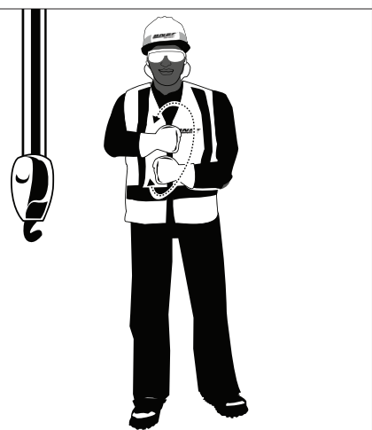
TRAVEL (Both Tracks): Use fists in front of body, making a circular motion about each other, indicating direction of travel, forward or backward. (For land cranes only.)
