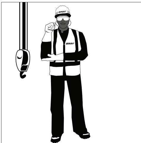
USE WHIPLINE (Auxiliary Hoist): Tap elbow with one hand; then use regular signals.
