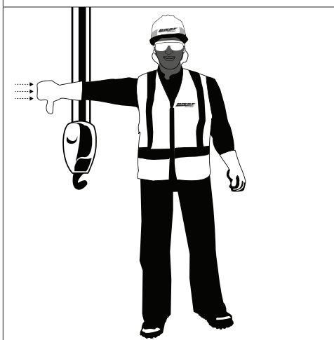
LOWER BOOM, RAISE LOAD: With arm extended, thumb pointing down, flex fingers in and out as long as load movement is desired.
