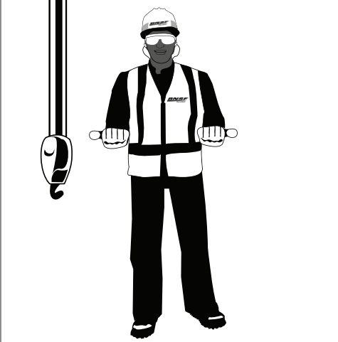
EXTEND BOOM (Telescoping Booms): Both fists in front of body with thumbs pointing outward.
