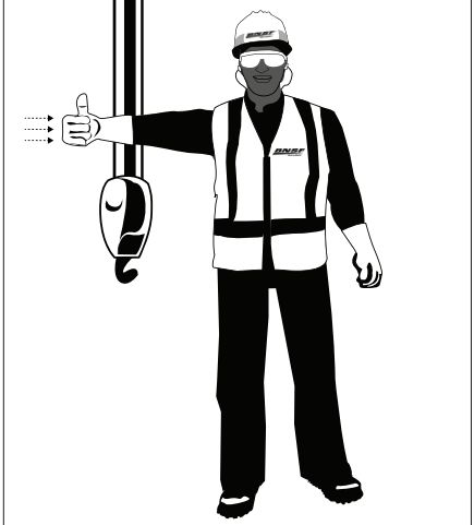
RAISE BOOM, LOWER LOAD: With arm extended, thumb pointing up, flex fingers in and out as long as load movement is desired.
