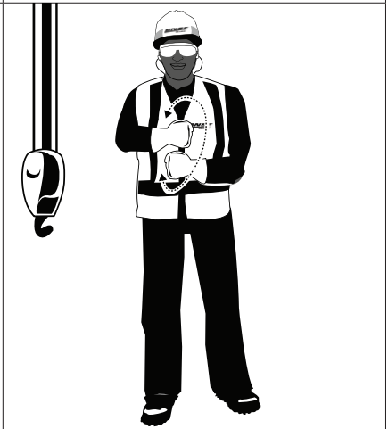
TRAVEL (Both Tracks): Use fists in front of body, making a circular motion about each other, indicating direction of travel, forward or backward. (For land cranes only.)
