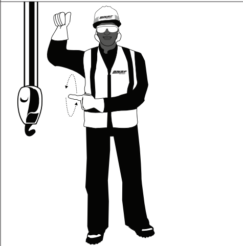
TRAVEL (One Track): Lock the track on side indicated by raised fist; travel opposite track in direction indicated by circular motion of other fist, rotated vertically in front of body. (For land cranes only.)
